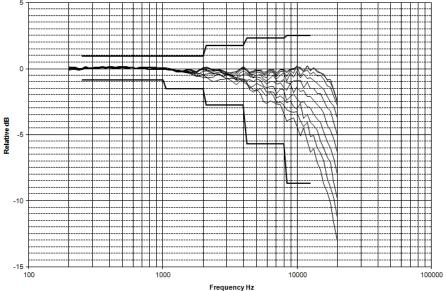
Directional frequency response positioned back toward noise source (0°-150°incidence angles)
